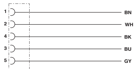
Contact assignment of the M12 socket
